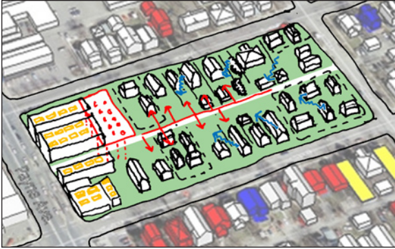
Improvements would include; district heating and cooling (red), solar (yellow) and stormwater management (blue)
